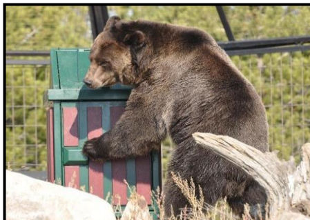
Figure 15. Photo demonstrates that the latch hood over paddle latch is smaller than bear paw to prevent the bear from reaching under the hood and activating the latch.
