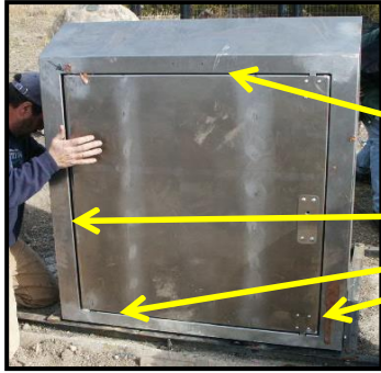
Figure 7. Garbage can enclosure showing gaps subject to measurement during technical evaluation.
