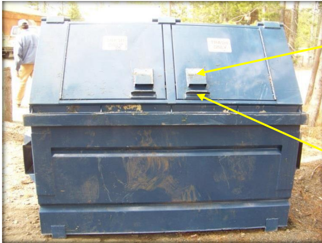
Figure 12. Bear-resistant dumpster showing latch hood and guard.
