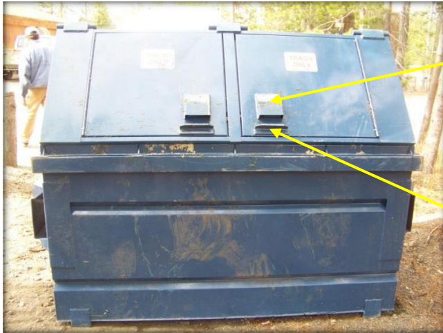
Figure 12. Bear-resistant dumpster showing latch hood and guard.
