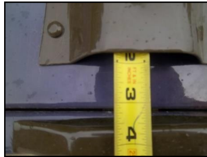
Figure 14. Example of distance needed between guard and latch hood opening. The tape begins at the latch (latch is located 2" inside hood).
